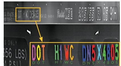
DOT-code is generated simultaneously from height data
