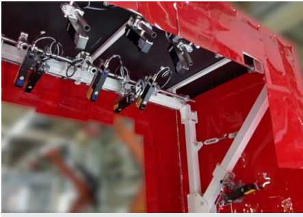
Bolting System with Gocator 3D Smart Sensors
