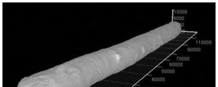
As the log moves through the scan plane, a full 3D map of the log surface is generated
