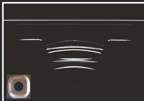
► A scan of a smartphone camera structure obtained using the FocalSpec LCI1201 line confocal sensor. In addition to dimensional measurements, particles and delaminated camera optics can be identified. ►
