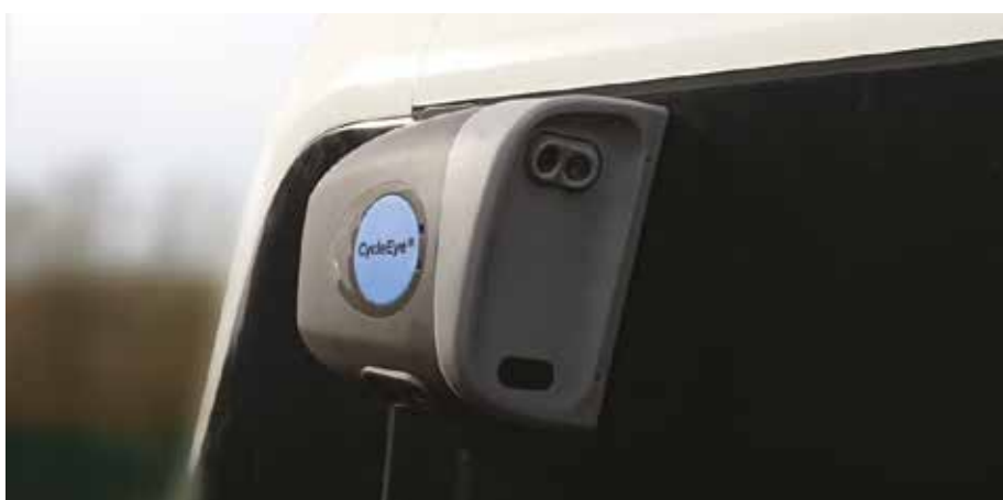
CycleEye CMS replaces wing mirrors on buses, combining HD cameras and radar to give the driver a view of what’s around the vehicle
