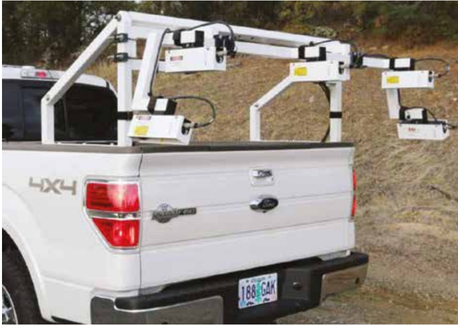
American highway officials are using a rig comprised of five LMI Gocator 2375 sensors mounted on a vehicle to measure the condition of pavements
