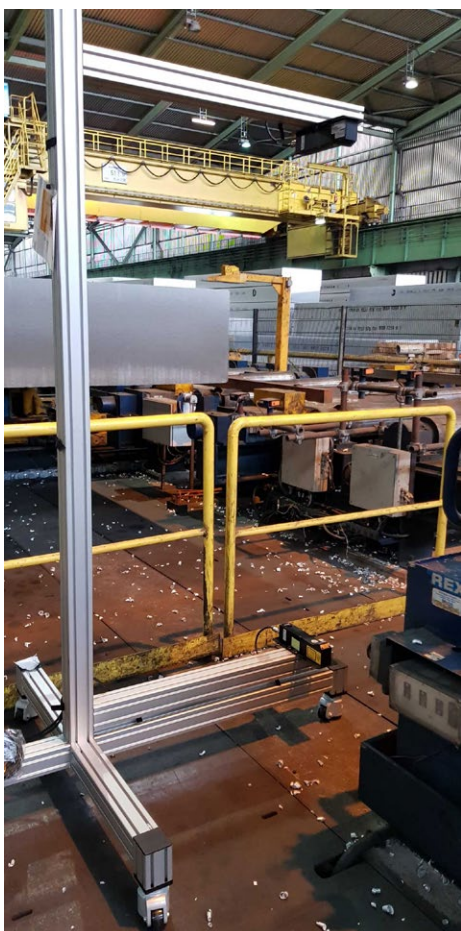
Custom bracket with 2 Gocator sensors for a simultaneous inline top and bottom surface scan
