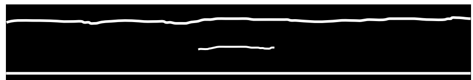
Tomographic cross section shows the thin air cavity as a third surface in the profile
