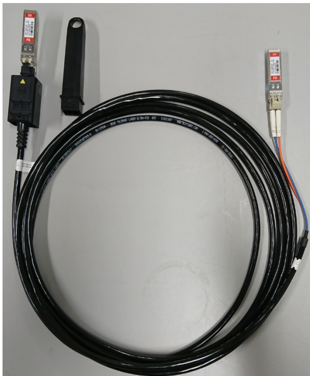
Figure 10. Optical cable with SFP+ modules in both ends
