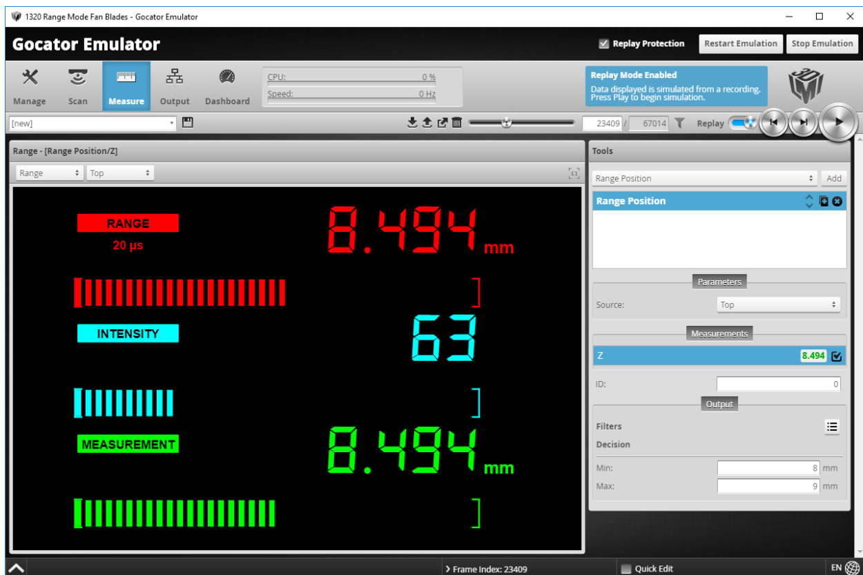
Emulator showing a range in recorded data. A measurement is applied to the recorded data.
