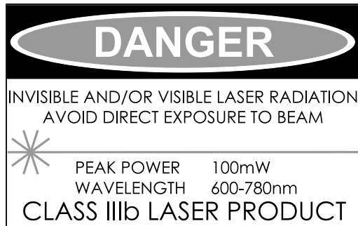
FDA warning sign example
