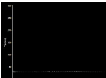
Under-exposure: Laser line is not detected. Increase the exposure value.
