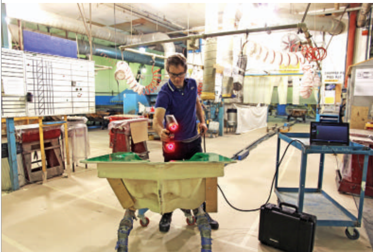
Creaform Inc.'s HandySCAN 3D being used in a laboratory environment.
