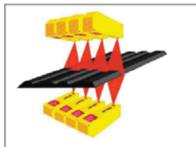
Fig. 2. For tire final inspection, three or more sensors are typically used.
