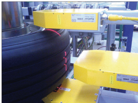
Fig. 3. A typical in-line automatic tire final inspection system.
