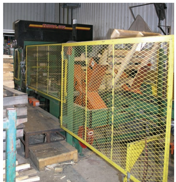
This Viking Turbo 505 pallet assembly line puts out 10 loads of pallets daily with minimal labour and risk. The company got its start in pallets, and today runs a separate division to supply Ontario's manufacturing heartland.
