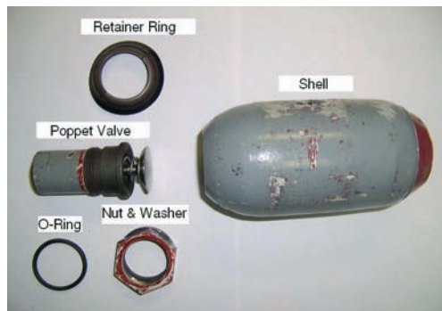
Figure 6. A breakdown of the accumulator, minus the bladder.
