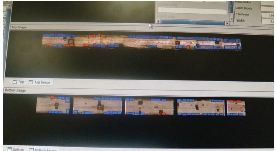
Knots are displayed on the Comact optimizer GUI.
