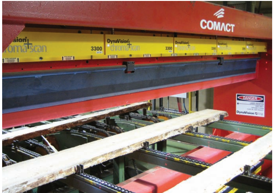
The DynaVision chroma+scan 3300 sensor from LMI Technologies can detect board defects earlier in the production process. The sensor is shown here installed on a Comact EdgeExpert system in the BC Interior. Photo: Courtesy Comact.
