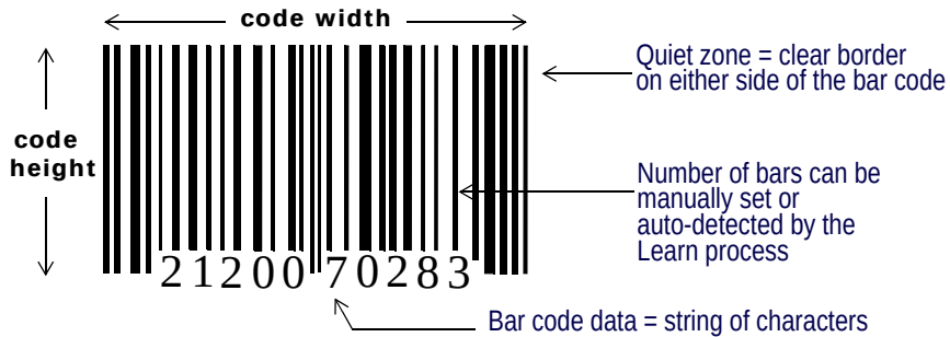
Figure 415 Elements of a Bar Code Symbology
