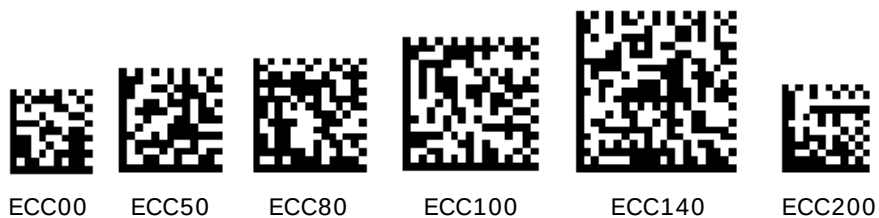
Figure 415 Data Matrix Examples with Different ECC Levels
