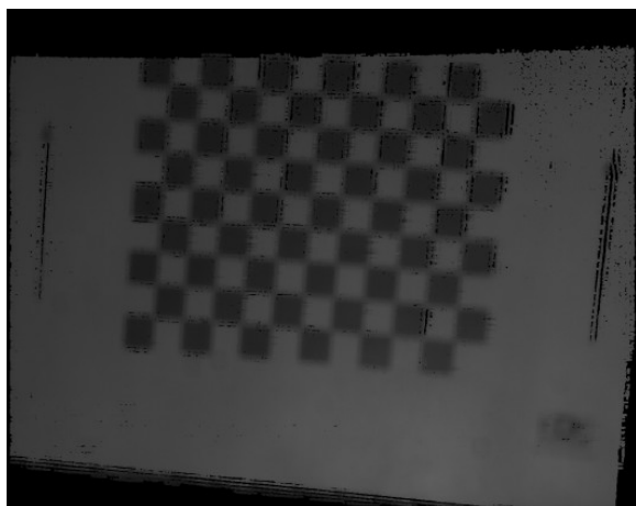
Single calibration, projector view, bad camera focus
