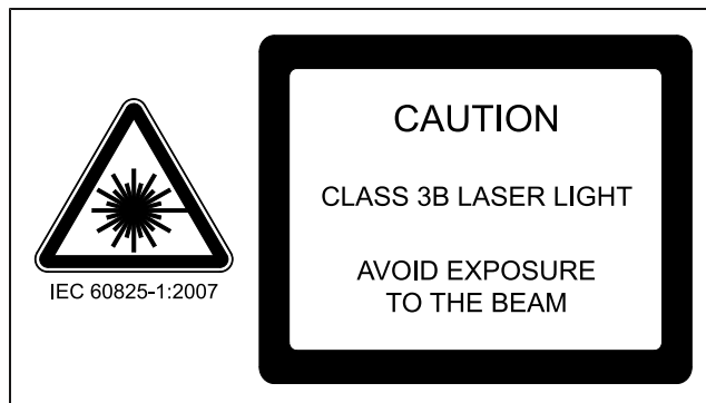
IEC warning sign example
