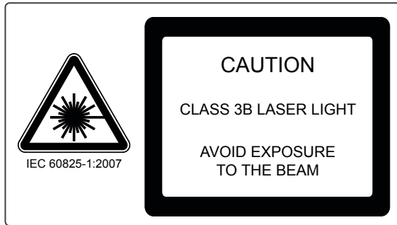
IEC warning sign example
