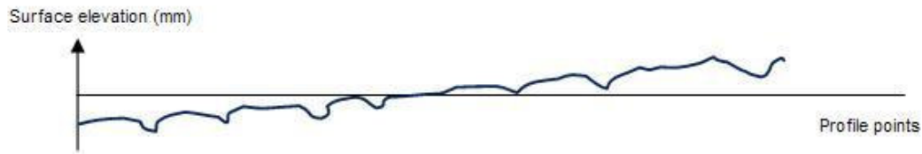
Figure 3.7.1: Raw Laser Line Profile
