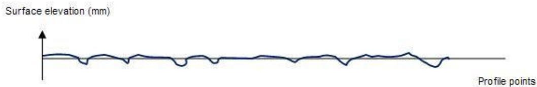
Figure 3.7.2: Laser Line Profile corrected for tilt.
