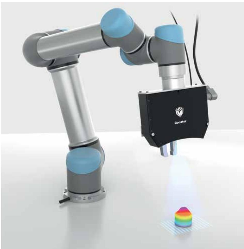
LMI's Gocator URCap plugin maps a Gocator snapshot sensor directly to a Universal Robots robot
