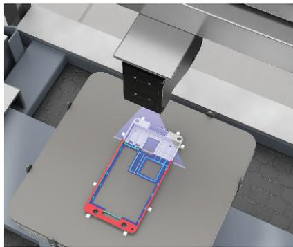
has a measurement range of 80mm and a wide field of view (48-100mm) for maximum scan coverage with fewer sensors.
