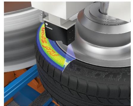
405-450nm of the visible light spectrum. Shorter wavelengths allow for a thinner, more focused laser line for precision measurements, create less speckle, and produce greater scattering. When scanning smaller surface features on highly polished and machined surfaces, the shorter wavelength and narrow laser line produce images with less noise, resulting in cleaner data.
