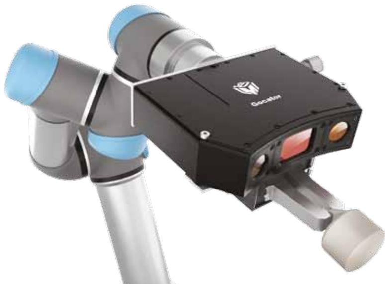
robot coordinates. This allows the position and orientation of an object detected by the sensor to be communicated directly to the robot. Critical X-Y-Z and angle information is communicated to the robot for use in vision guidance, inspection, and pick-and-place applications.
