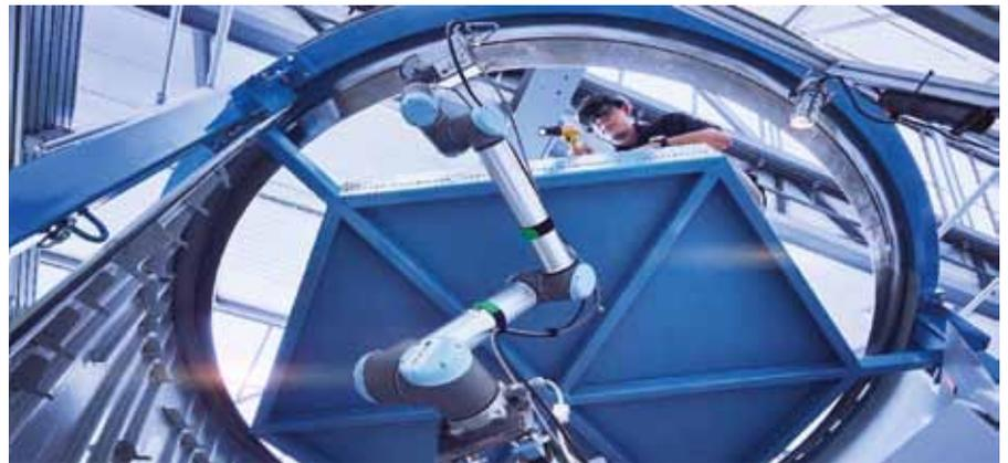
Tasks in the riveting process are divided between human and robot. The human detects the designated hole, inserts the rivets, positions the riveting hammer and starts the collaborative process by activating the hammer. In parallel, after ascertaining the position of the holes, the robot positions the anvil and bucks it against the rivet during the execution of the process.
