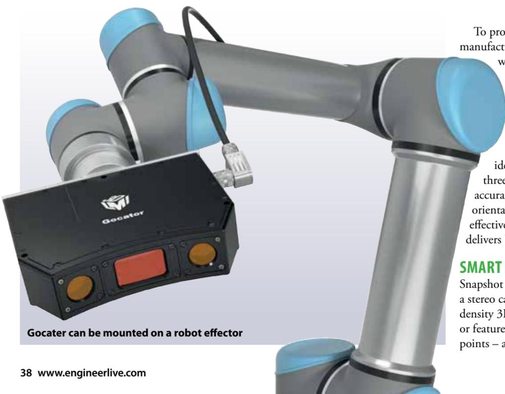
Gocator can be mounted on a robot effector
