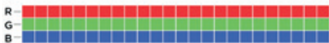
Figure 3: Trilinear cameras offer three pixel rows, or, one for each R, G, B colour
