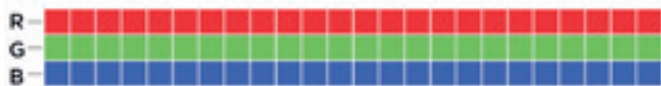
Figure 3: Trilinear cameras offer three pixel rows, or, one for each R, G, B colour
