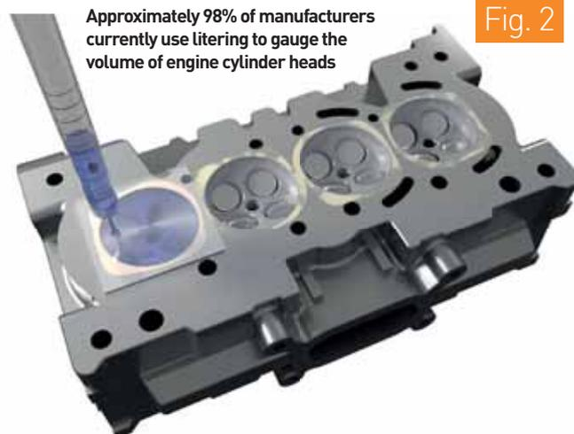
Approximately 98% of manufacturers currently use litering to gauge the volume of engine cylinder heads
