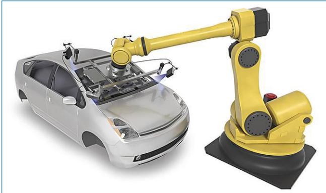
Vision guidance is critical for many robotic assembly applications, such as windshield installation. Photo courtesy LMI Technologies Inc.
