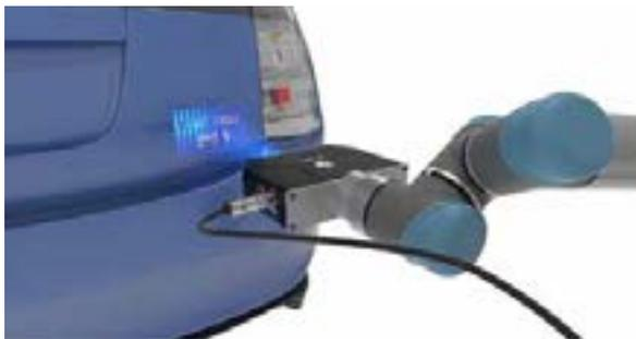
*Fig. 8 Badge inspection using Gocator 3210 snapshot sensor mounted on a robot arm.*
