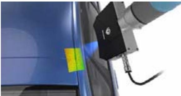
*Fig. 4 Gap & flush measurement using a Gocator 3210 snapshot sensor mounted onto a robotic arm.*
