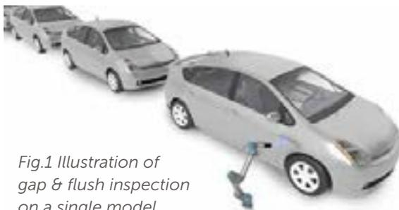
*Fig.1 Illustration of gap & flush inspection on a single model production line.*
