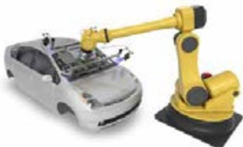
*Fig. 3 Windshield insertion using a vision-guided robotic arm.*
