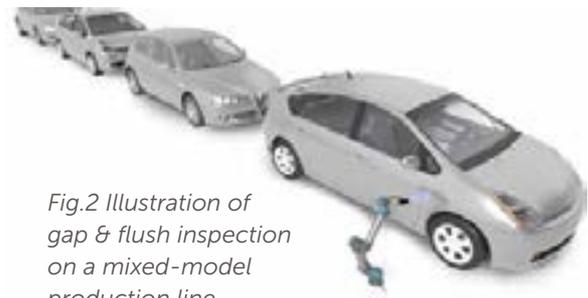
*Fig.2 Illustration of gap & flush inspection on a mixed-model production line.*
