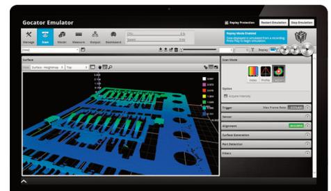
Emulator allows you to perform 3D measurements on pre-recorded data taken from actual scanned objects (in this case, a small electronic part)
